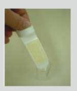
Dipslides have a typical shelf life of 8 - 9 months. Once the dipslide is opened care must be taken not to touch the media or expose the media to the atmosphere in order to prevent false contamination.
